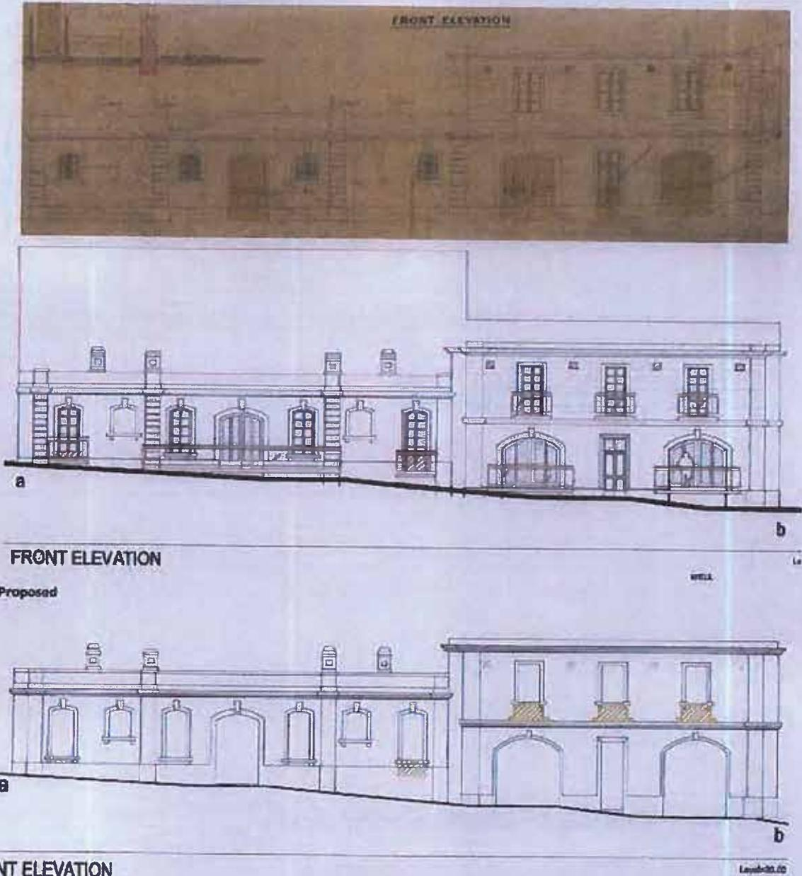
Figure 9: Comparative study of Proposed/ Existing Elevations with Historic Elevations
